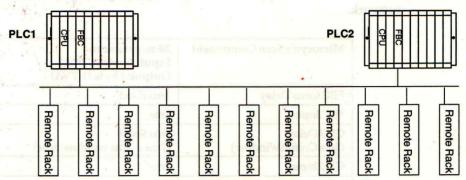
CPU utilization is much higher in this example. This is mainly because there are fewer I/O scan operations between the CPU and the FBC during the same unit of time. With fewer I/O scan operations, more time is available for logic solution in the PLC CPU.
